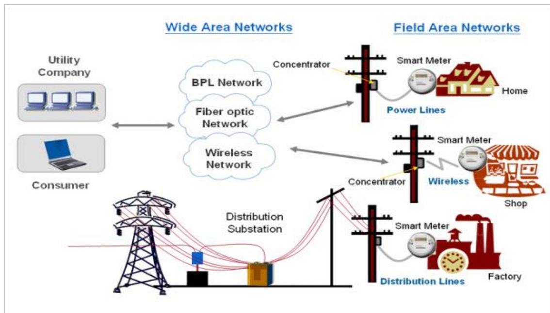
Figure 2.4: A typical Advanced Metering Infrastructure
